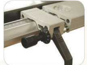
Micro fence setting scale to within 1/10th mm calibrations.
